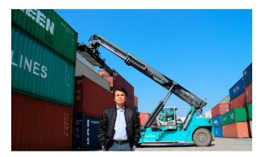
equipment, their third purchase was an SMV 4531 TCE5 in September 2019, a next-generation reach stacker that adds even more power with a sturdy, box-type chassis, a wide drive axle and a long wheelbase for high stability and safe handling.
