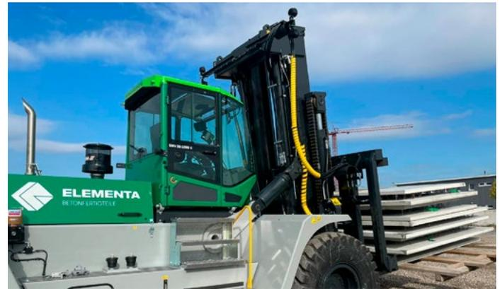
It also includes a range of features such as individual fork positioning, auto engine, lighting and ignition shutdown, and a height indicator laser, as well as the latest fuel-efficient engine for less exhaust emissions, compliance with tough EU environmental regulations, and reduced noise.
