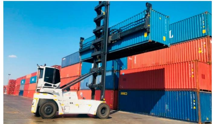
Fitted with a spacious cabin and ergonomic controls, each lift truck provides drivers with large, lowered front windows without corner posts, for excellent visibility in all directions. Special features such as smart load sensing as well as Electronic Machine Control (EMC) for automatic engine shutdown and speed limit combine for better fuel efficiency, safety, and durability across a long life cycle.
