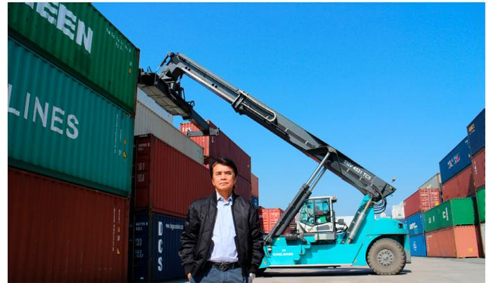
equipment, their third purchase was an SMV 4531 TCE5 in September 2019, a next-generation reach stacker that adds even more power with a sturdy, box-type chassis, a wide drive axle and a long wheelbase for high stability and safe handling.
